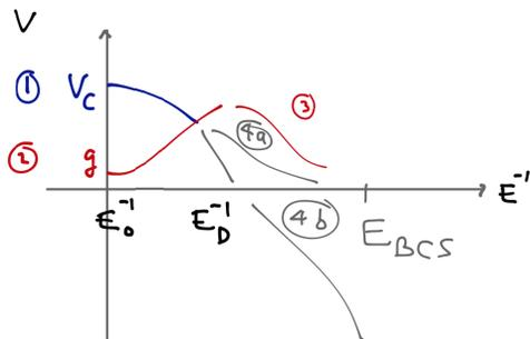
Here's the narrative, proceeding as a function of decreasing energy scale, beginning at  $E_0$ , the Planck scale of solids: (1) Electrons repel each other by the Coulomb interaction. However, in a metal, this interaction
