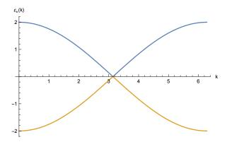
which is the single band  $\epsilon(k) = 2\cos 2k$  folded on itself into the smaller Brillouin zone. In this case, the system is a metal, since we must fill up half the band.
