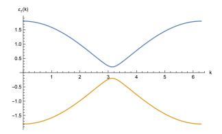
The system is an insulator, since we fill the bottom band, and then the energy cost to excite an electron in the upper band is
